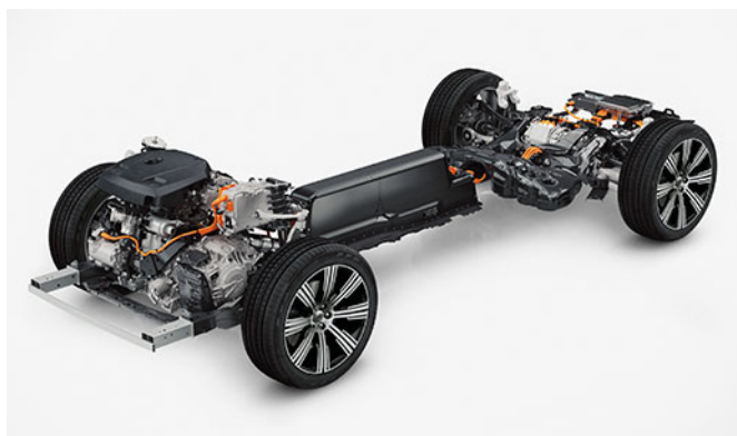
The battery's location helps give your Volvo a low centre of gravity, so it is stable, sure-footed and comfortable while not affecting the car's load space.
